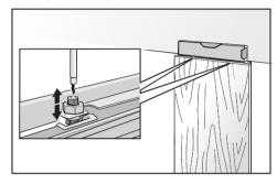
■ Align the door to the side by sliding it over the threaded bolts.
